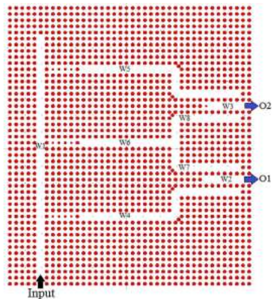
Fig.14 ADC with three nonlinear resonant cavities [91].
