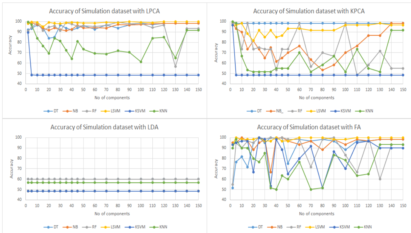
Figure 5: The accuracy of different classification techniques applied with each reduction technique on Simulation dataset
