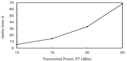
Fig. 8. Signal quality factor in relation transmitted power.
