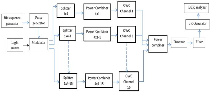
Fig. 1. B. Simulation Model 16 TX/RX IsOWC system.
