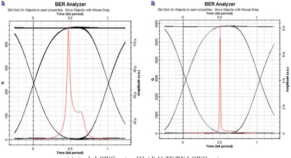
(c) simple IsOWC system [1] (d) 16 TX/RX IsOWC system Fig. 4. Eye diagram of the simple and 16 Tx/RX IsOWC at wavelength 950 nm.
