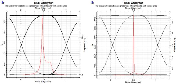
(a) simple IsOWC system [1] (b) 16 TX/RX IsOWC system Fig. 3. Eye diagram of the simple and 16 Tx/RX IsOWC at wavelength 850 nm.
