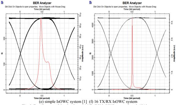
Fig. 5. Eye diagram of the simple and 16 Tx/RX IsOWC at wavelength 1310 nm.
